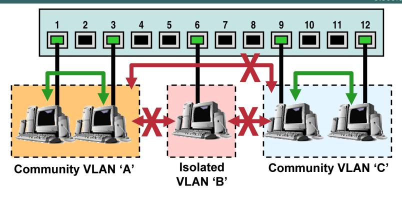
...Private VLAN's allows the creation of "sub-VLAN's" within a primary VLAN. These "sub-VLAN's" known as community VLAN's and Isolated VLAN's restrict the movement of traffic while allowing the use of the same subnet address space. Communication outside of the "sub-VLAN" Can only take place via the promiscuous port...
